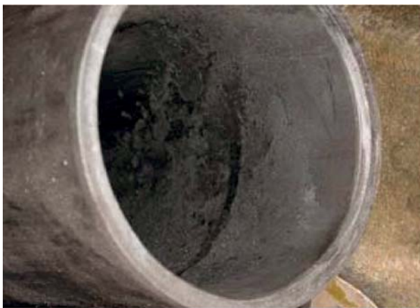
Figure 04b: Typical deposits of inner diameter of valve guide (MC70-type after 8,200 hrs)
