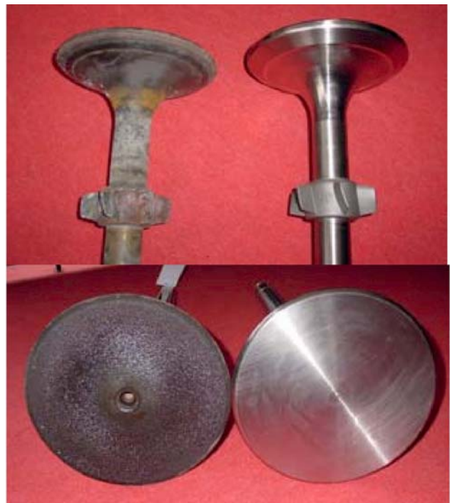
Figure 15 a/b: Nimalike spindle before and after remanufacturing
