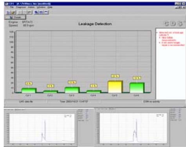
Figure 18: Documentation of the result of leakage detection and valve timing/ignition
