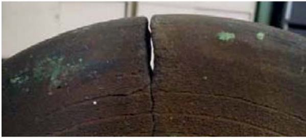
Figure 14: Failure of a valve spindle (RTA84 Nimonic type 5, 270 hrs after repair).
