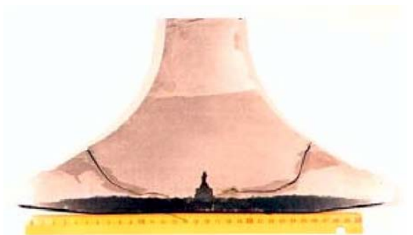
Figure 13: Macro cut through the center of a valve head (RTA62 Nimonic-type 6,430 hrs after repair)
